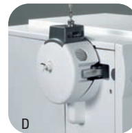
C Use the PhotoMate APPI source to ionize samples that respond poorly or not at all with APCI and ESI.
