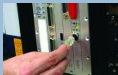
Ethernet connectivity transmits data from the spectrometer's fully digital components to the OPUS software. The plug-and-play electronics brings ease-of-use to FT-IR spectroscopy.
