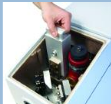
The dual DigiTect™ detectors provide superior performance and allow easy manual exchange by the user.
