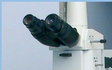
The RAMANSCOPE ™ FT-Raman microscope for non-destructive analysis of microscopic samples
