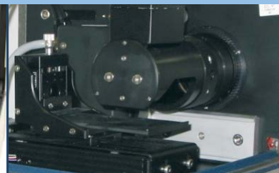
Motorized horizontal sample video stage for high sample throughput and Raman mapping
