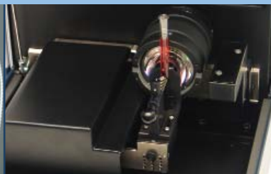
Large sampling compartment holds various prealigned sample stages and other accessories
