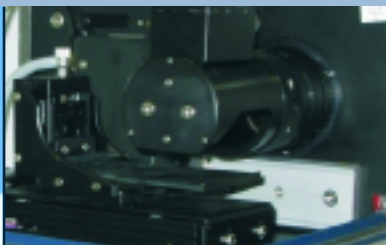
The horizontal video sample stage provides convenient sample handling and visualization.
